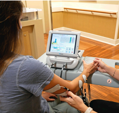
Xcite2 Clinical Station, a mobile functional electrical stimulation (FES) therapy device
